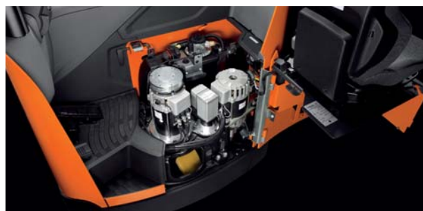
BT Reflex has durability designed-in with its sealed electrical units, brushless motors and leak-free connectors
