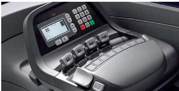
Standard mini-levers allow fingertip control of each fork movement
