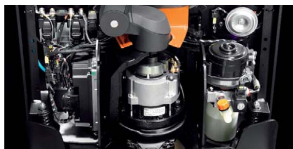
The fixed motor has no moving cables
